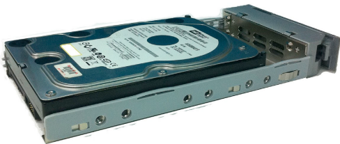
Figure 12: SAS disk drive mounted in a drive carrier
