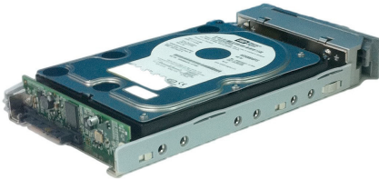
Figure 14: SATA disk drive mounted in carrier with AAMUX adapter
